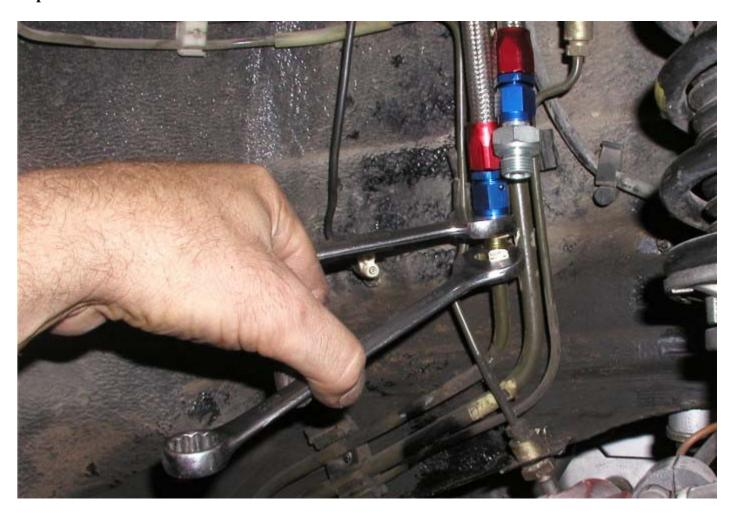
Having made sure the steel fuel line has not slid down from inside the fitting, do a final tighten of this connection.
