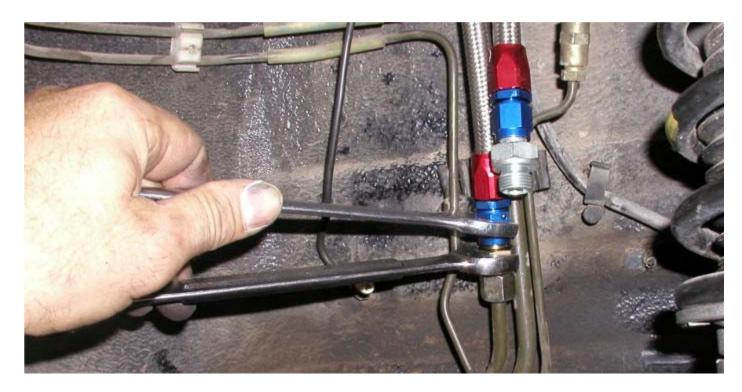
Final tighten the fuel lines end fitting (blue in this picture) to the compression fitting.
