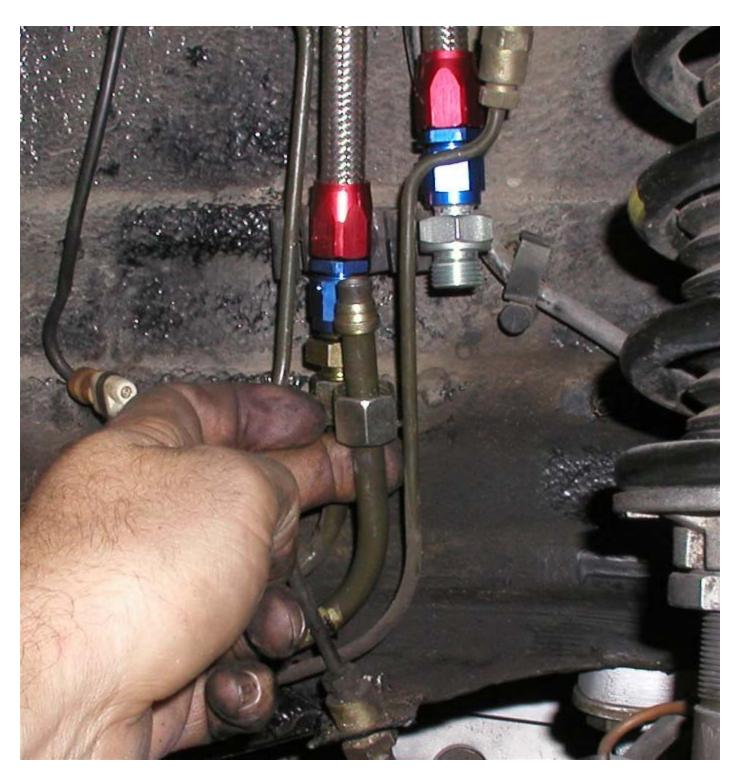
Here you see we have cut the 10mm steel line at our mark, and installed the 10 compression nut and 10mm bite sleeve as we did with the 8mm return line. Same process on this line.
