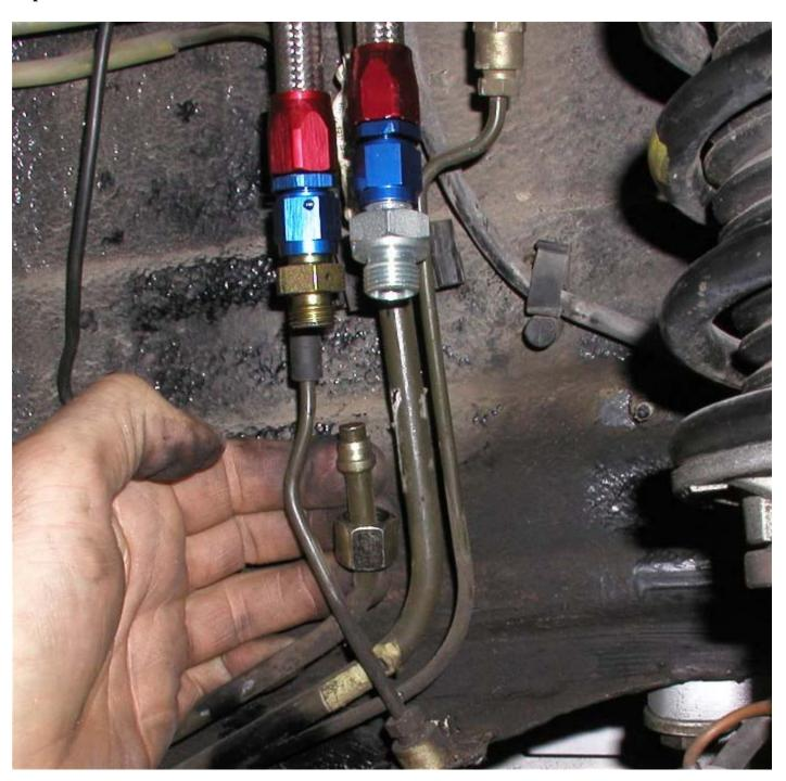
Here we have slipped the 8mm compression nut down the 8mm fuel line. Then slide down the "bit sleeve" in this orientation. Fat end down! We want to see steel line protruding out the bite sleeve as pictured.
