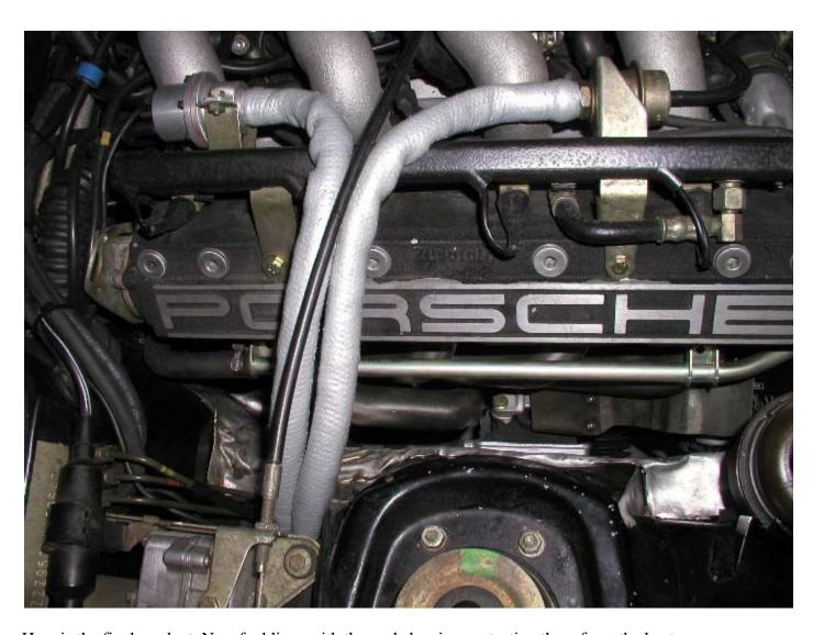
Here is the final product. New fuel lines with thermal sleeving protecting them from the heat.
