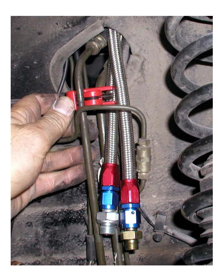
On this particular car, it has ABS which means it has many more brake lines around the fuel lines. Some of these make the job difficult. The mark to cut the lines is actually further down the steel tube. Here we are cutting the lines near where the brake line crosses over the fuel line to allow us to then swing the fuel line out from behind the brake line to make it easier to make your cut down low at the actual marked spot.
