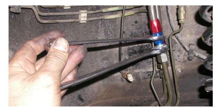
Final tighten the compression nut to the compression fitting.
