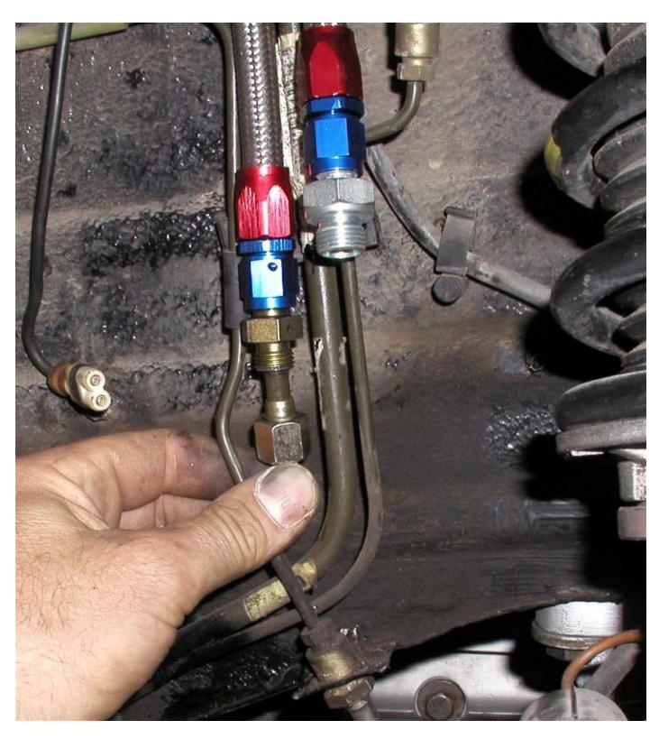
Although we could not accurately show it, because one hand was holding the camera, hold the compression fitting that is attached to the new fuel line down against the new cut off 8mm steel line. The steel line should be going up inside the compression fitting about 10mm. Then while
