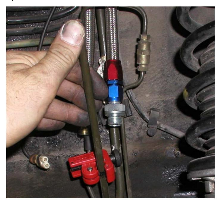
Here we are making the final cut at the marked spot on the return fuel line. You can rotate or lean the fuel line out having made the upper cut first making it easier to rotate the tubing cutter
