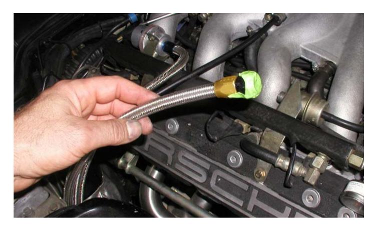
On this installation, we are going to install the optional Thermal Sleeving on the fuel lines. Since the sleeving is fiber lined, we are concerned about these fibers getting into the fuel lines when sliding the sleeving over the fuel lines. So we put a piece of tape temporarily over the end of the line to seal it. This will insure we don't clog a fuel injector.
