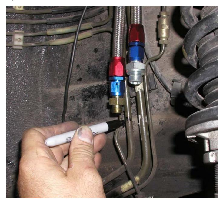
Temporarily install (hand tighten) the supplied compression fittings on to the new replacement lines. The 10mm compression fitting on the 10mm (front) feed line, and the 8mm compression fitting on the 8mm (rear) return line. You can look at the compression fitting and determine which is the 10mm and 8mm by visual size comparison. The opposite end of the fitting is the same.
