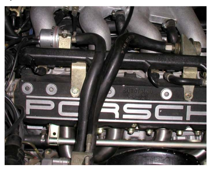
These are the stock fuel lines we are about the replace on a 944 Turbo. Late 944s, where the fuel line enters through the shock tower, are essentially the same. For future reference, the front line (right on picture) is the high pressure fuel feed line to the fuel rail. The rear line, (left in picture) is the low pressure return line back to the gas tank. The feed line is 10mm in diameter where
