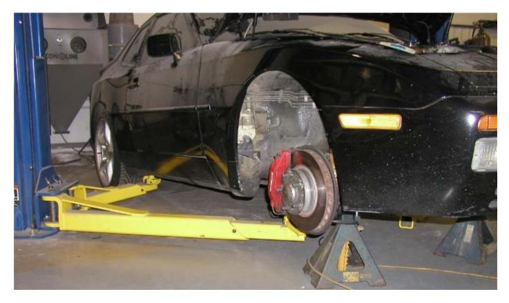
We need the front of the car raised up and the rear of the car down. We do this so, when we cut the fuel lines, you will not have fuel continually running out of the lines onto the floor, which would be a fire danger.
