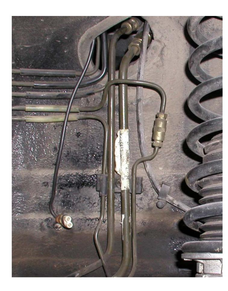
Here you see the 10mm feed line (right) and the 8mm return line (left) view from the wheel opening with the plastic inner fender removed.
