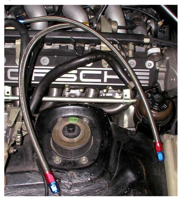
Disconnect the factory fuel lines at the fuel damper and fuel regulator and move them slightly aside. Then attach the new replacement lines at the fuel damper and regulator.
