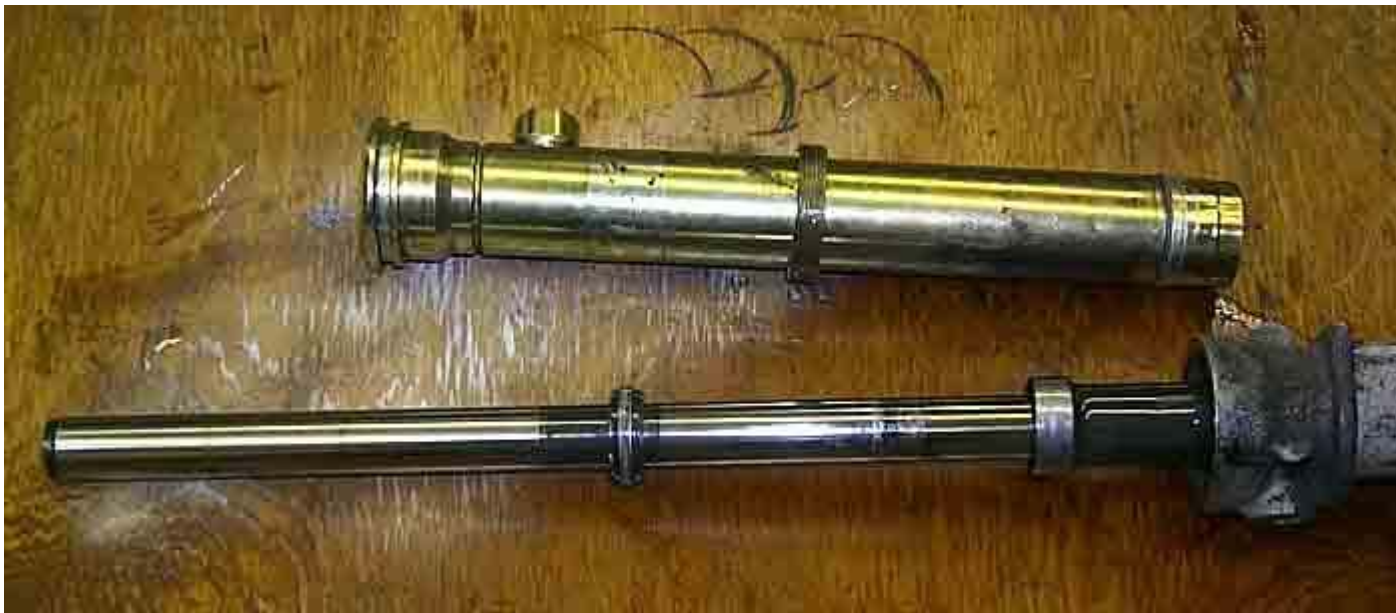
This is the rack housing removed from the rack.
