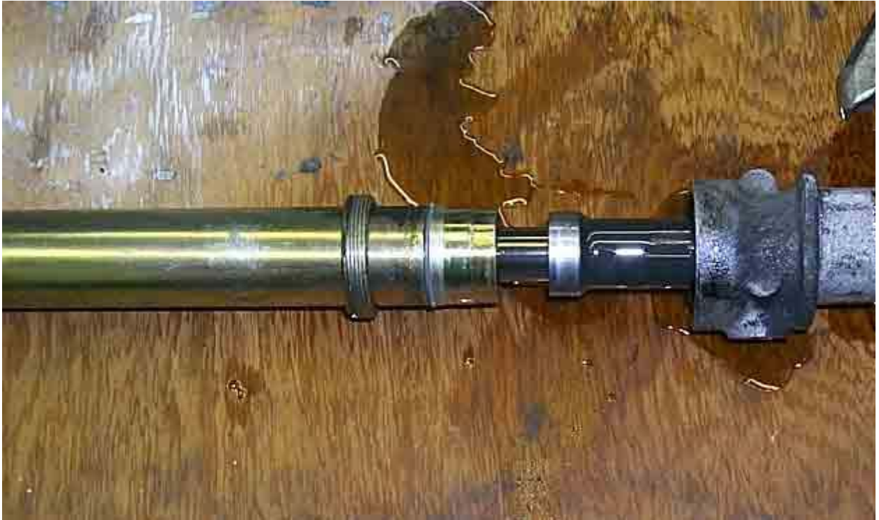
Here is the rack after the ring has been removed and the rack housing has been slid back.
