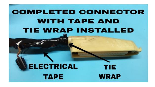
Step 6: Once you have double checked all of your work you can now reconnect the vehicle battery and start the vehicle. Add additional tie wraps to secure the new harness to the engine wiring harness as needed.
