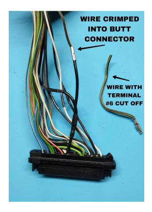
Step 10: Lay the wires flat in the KLR connector and install the connector back into the connector cover. The back of the connector needs to be inserted first. When installed properly, the connector will sit flush with the face of the connector cover. Install the screw into the connector. Apply electrical tape to the base of the connector where the rubber boot was removed and tape up the harness. Reconnect the KLR connector to the KLR.
