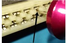
TERMINAL RELEASE TOOL INSTALLED IN CONNECTOR
