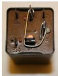
4. Jumpering these terminals and starting the car may also be used as an indirect method of testing the DME relay if a multimeter is unavailable. In other words, if the car will not start and you suspect the DME relay, install the emergency jumper and attempt to start the car. If it starts normally, it's very likely that the DME relay is bad.
